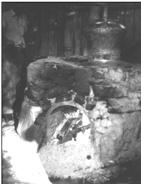
Photo 5: A typical modern still enclosed within a very substantial stone-built ‘corlon’. The copper lid or ‘capac’ in the shape of a ‘comanac’ can be seen: also the fire and the wood fuel consisting of tree branches. Photographed at Mușcel near Pătârlagele
