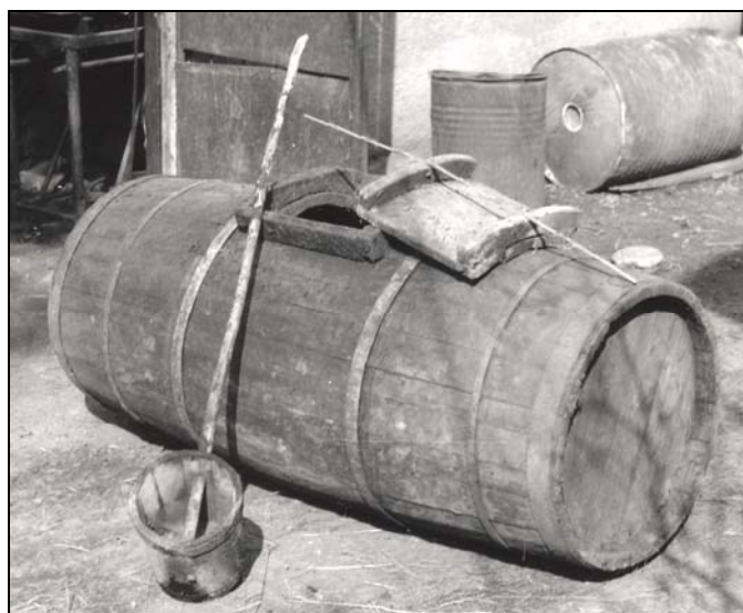
Photo 4: A ‘borhot’ may be transported to the still using a ‘cărător’. Note the bucket (‘ciolmic+’) with a long handle used for charging and discharging; also the large square opening or ‘gaură’ in the ‘cărător’ that must be provided by cutting through three of the curved staves. The picture was taken at Constantin Butucă’s distillery in Pătărlagele and shows empty metal drums that are frequently used as the ‘corlon’ for a small still or a ‘răcitor’ (condensation vessel)
