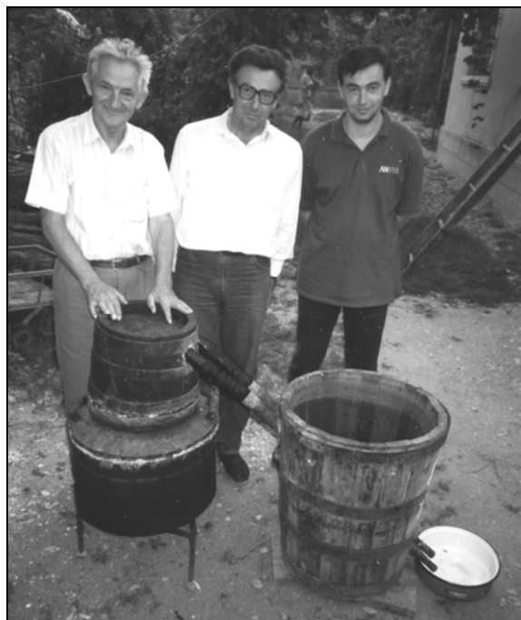
Photo 8: The traditional distillation system maintained for a small family operation at Bălcești/Ghioroiu (Vâlcea). The small copper still is fitted with a wooden ‘capac’ (albeit one constructed from staves with iron hoops like a small inverted bucket). Two copper pipes pass through the condensation vessel while a domestic kitchen pot serves as a spirit receiver. The leader author is pictured with the householder and his son
