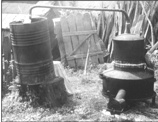
Photo 6: A typical small still using the modern system at Mușetești near Târgu Jiu (Gorj): the ducts for charging with ‘borhot’ (‘incărcător’) and discharging ‘boască’ (‘descărcător’) are clearly visible (especially the latter); also the horizontal pipe (‘cumpană’, but usually ‘cocae’ in Gorj) leading to the condensation ‘spiral’ contained within an oil drum. All the equipment is easily transportable: note the handles on the still and the ‘capac’. The latter is removable and hence the joint must still be sealed before operations commence although the use of metal for both the still and the lid ensures a tight fit with little distortion. Unlike the situation in Plate 5, there is no proper grate and the fire is not so easy to control
